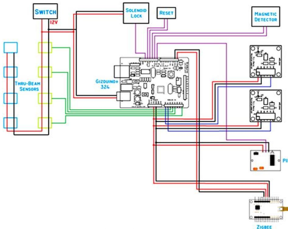
Figure 9. Interfacing of sensors to the microcontroller
