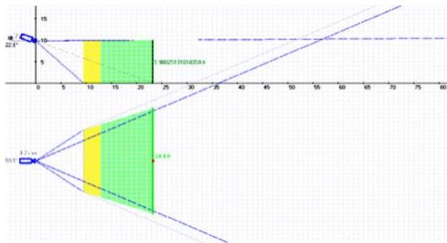
Figure 7. Camera height installation, tilt and viewing angle
